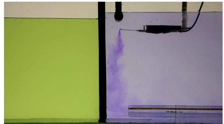
Unstable air curtain installation ( D_m \lesssim 0.1 )
