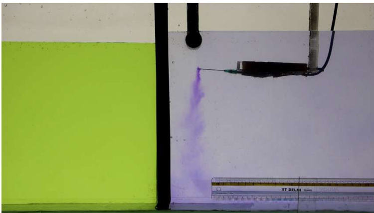
Stable air curtain installation ( D_m \gtrsim 0.2 )
